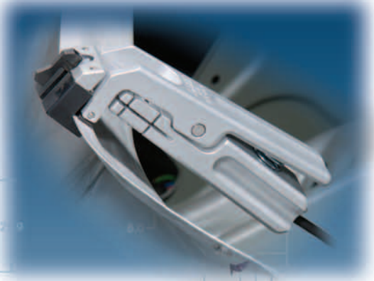
LMI 238 Deck Lid Seal Gap Gauge
