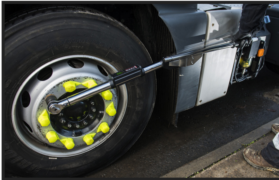
An SB750S breaking over at set torque
