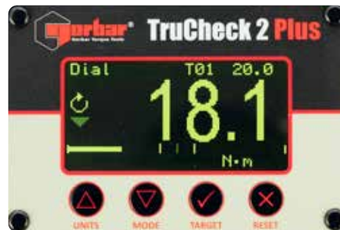
TruCheck™ 2 Plus display showing below target tolerance
