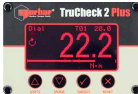
TruCheck™ 2 Plus display showing above target tolerance
