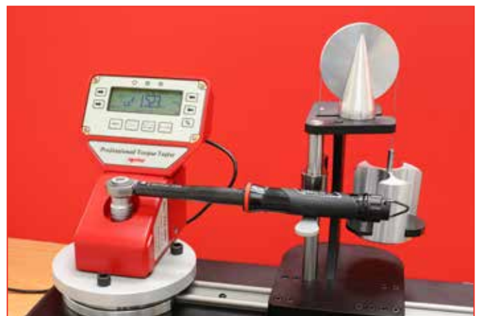
60323 Pro-Test and Static Torque Block Adaptor Kit
