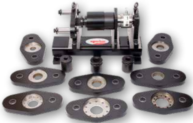
Power Tool Test Rig with Reaction Plates (50800)
