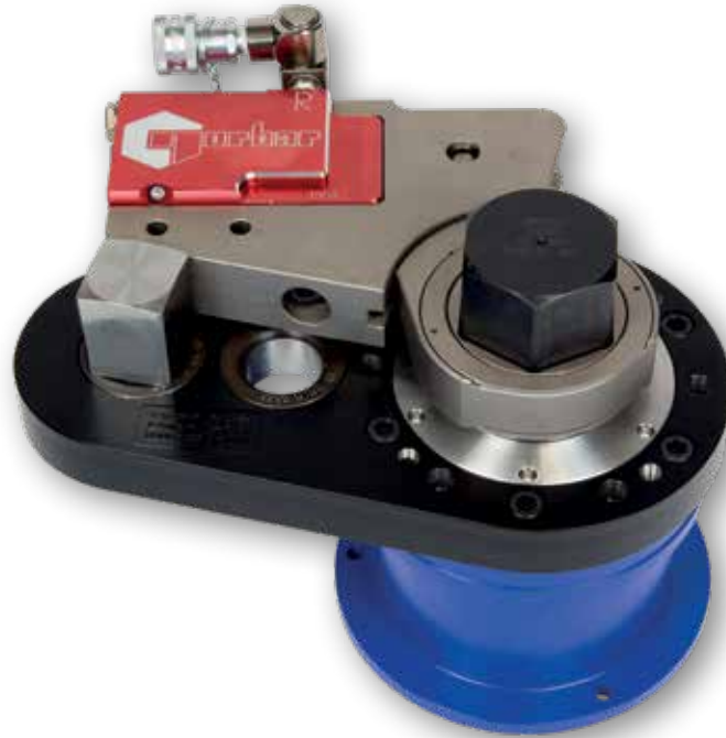
Fixture shown with Hydraulic Torque Wrench
