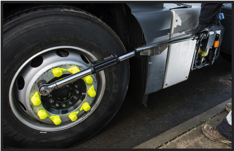
An SB750S breaking over at set torque
