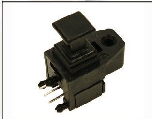
OTJ-2/ORJ-2 Single Optical Transmitter and Receiver Jack. Right angle PCB mount with self tapping hole for panel mounting. Removable plug-in cover.
