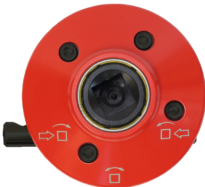
AWUR set to counter-clockwise operation
