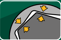
Sockets feature off-corner loading
