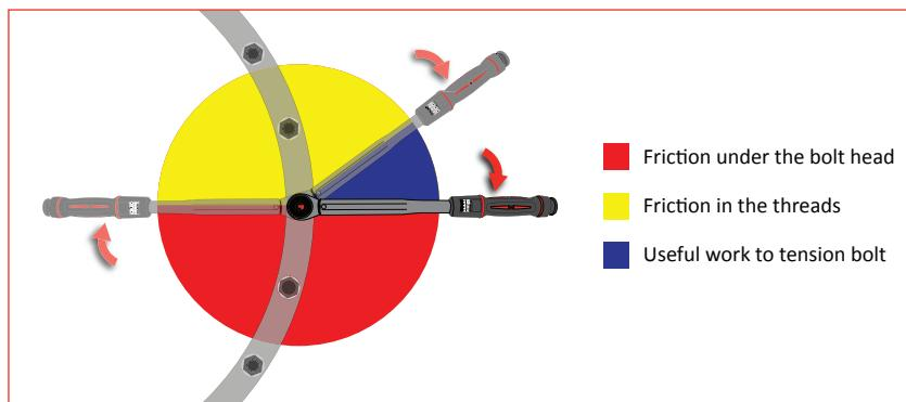
Given that up to 90% of the applied torque will be lost to friction, it follows that any changes in the coefficient of friction resulting from differences in surface finish, surface condition and lubrication can have a dramatic effect on the torque versus tension relationship. Some general points can be made:
