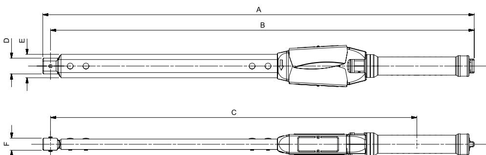
NOTE: When using the Extension Handle (14142) add 495 mm to dimensions 'A' and 'B', add 515 mm to dimension C and add 1.6 kg to the weight.
