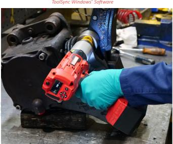
Brake Actuator for a underground train
