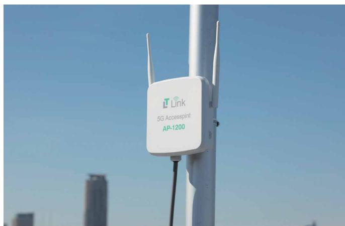
ASA material is resistant to deterioration and discoloration due to ultraviolet rays. Perfect for outdoor communication or network devices.
