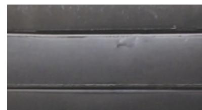
**EPDM material from weatherproof cable gland of another manufacturer :** Cracked, color drastically faded and powder appeared on the surface.
