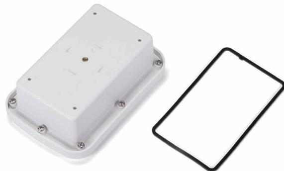
With a silicone waterproof gasket, and supported by multiple enclosing screws from the rear side, it allows the enclosure to maintain a stable high waterproofing capability.
